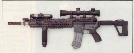
Here Johnston's rifle is seen with the ACE SOCOM 16 retractable stock, ERGO pistol grip and the Grip-Pod vertical foregrip/bipod. Fully equipped, the "Mk 12 Mod 2" weighs in at about 9.5 pounds.
